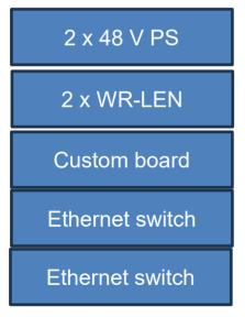
Custom board to convert WR-LEN to custom timing and to be a patch panel for connection and similar
