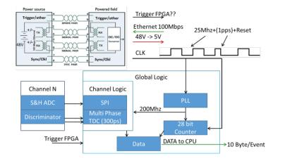
We can decide to add the necessary hardware, so DAC (like AD5662BRMZ-1) and clock generator CDCM61004RHBT, to the existing board or we can decide to use a standalone mezzanine to speed up the development, like the one developed for LHAASO.
