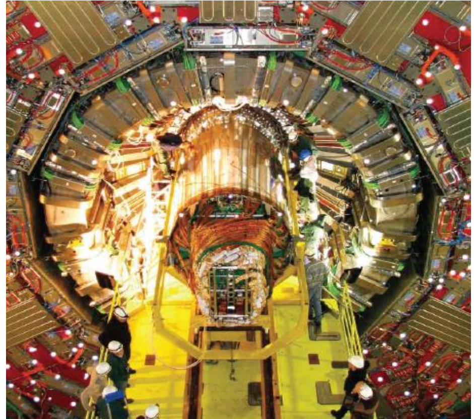
insertion of the CMS Si tracker; a few people stand by, operational 2008-now
