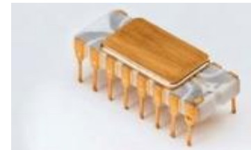
1971 Intel 4004 10 \mu\text{m} nMOS
