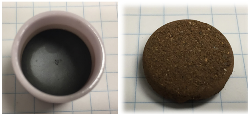
Fig. 2. a) Lunar Mare simulant heated to 1500 °C for 3 h with argon purge, b) heated to 1100 °C for 3 h with argon purge.
