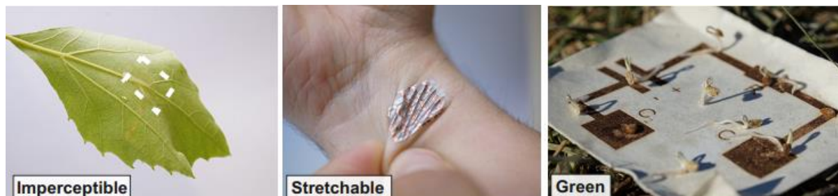
Flexible Electronics with different functionalities (from left to right): transparency, mechanical flexibility and biocompatibility.
