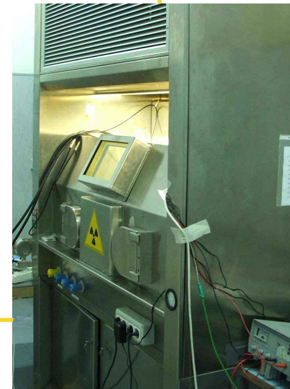
$^{7}\text{Be}$  (and Li) deposited into source cathodes, typically 1.5 GBq each
