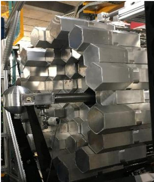
Tagging detector for Fusion-evaporation and direct reactions with n ejectiles
