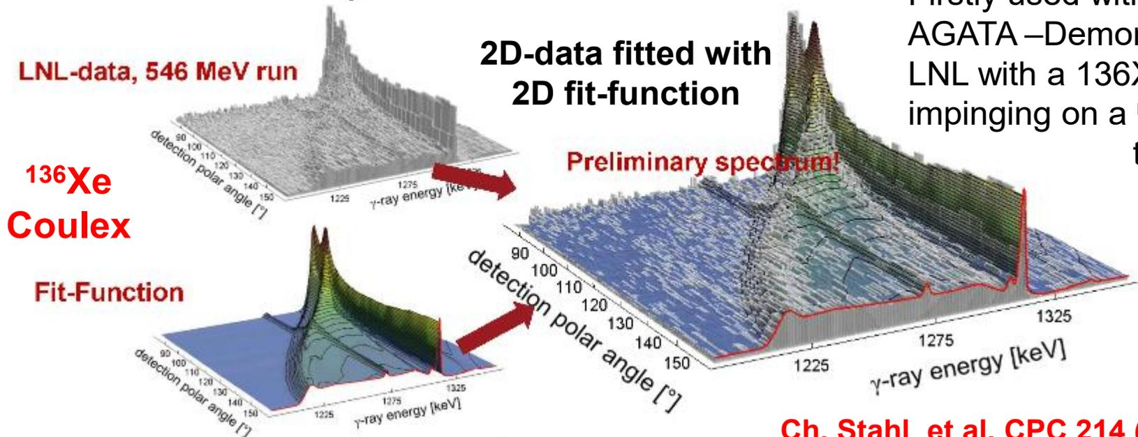
Firstly used with the AGATA – Demonstrator at LNL with a  $^{136}\text{Xe}$  beam impinging on a  $^{\text{nat}}\text{C} + \text{Ta}$  target.
