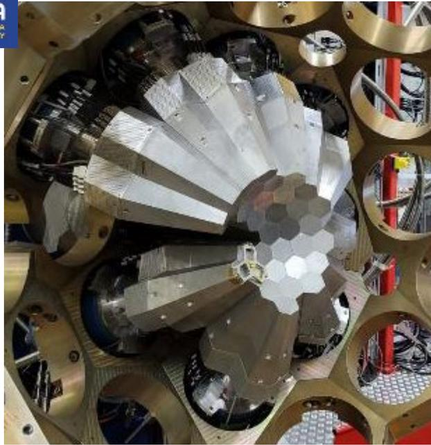
AGATA is the High-Resolution **flagship instrument** in Europe for completely characterizing the **structure of exotic nuclei** by measuring **excitation energies, spin & parity, lifetimes, static moments, exclusive cross sections, etc.**
