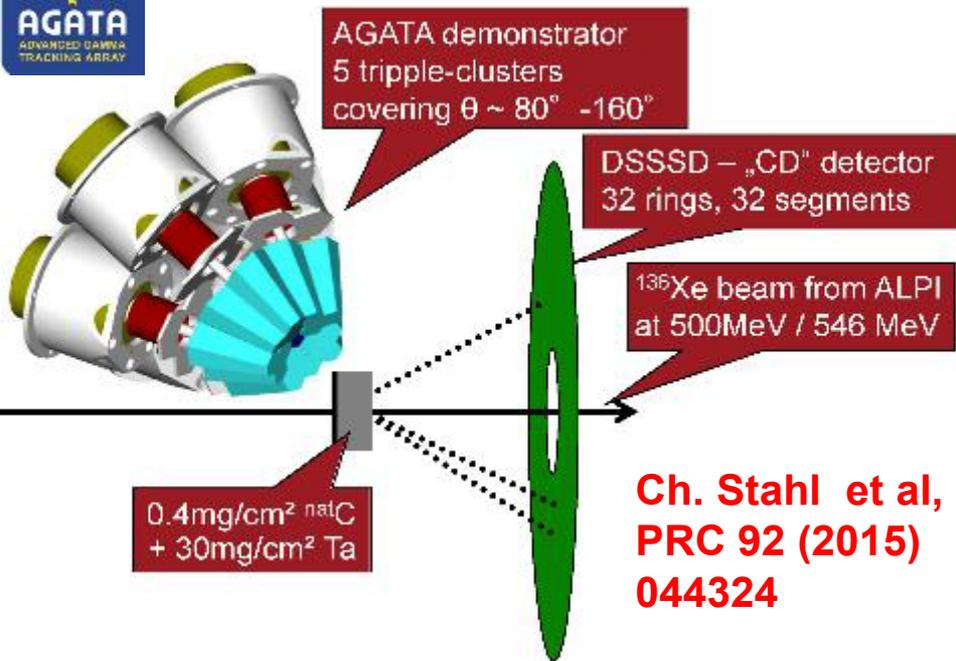
The continuous-angle DSAM represents an advancement of the “conventional” DSAM. It extends the  $\gamma$ -ray lineshape analysis as a function of  $\gamma$ -ray energy to a lineshape analysis as a function of both  $\gamma$ -ray energy and polar angle of the  $\gamma$ -ray detection.
