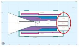
The collimator is taking out a fraction of the particles going from Production Solenoid to Transport Solenoid.
