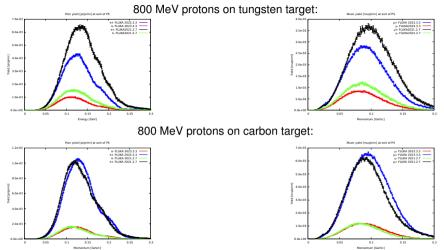
Results do not change much for carbon target design, but are lower by  $\sim$  30% for tungsten target - reason has probably been understood (**not** due to a change in **FLUKA** physics, but geometry had been changed for tungsten target).
